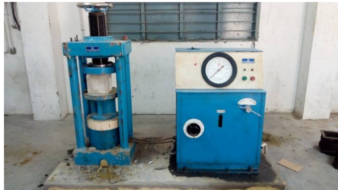
Fig No: 2 Compression test on cubes
